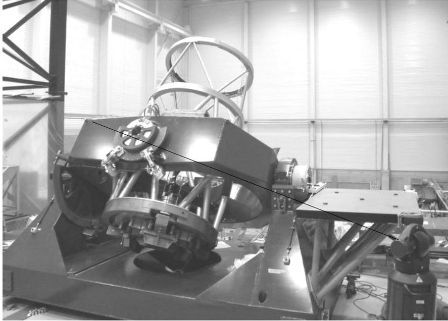
Figure 4. Main axes measurement by means of the laser tracker (laser beam sketched over the picture)
