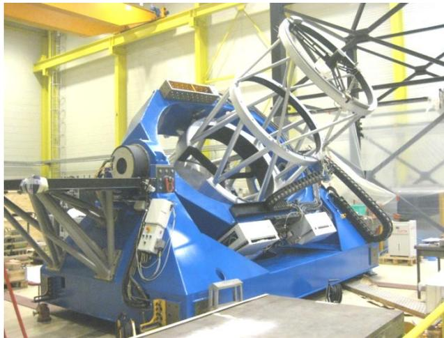
Figure 4 - The MROI elevation over elevation 1.4m UTM under test at Vendor's facility (Courtesy of AMOS).
