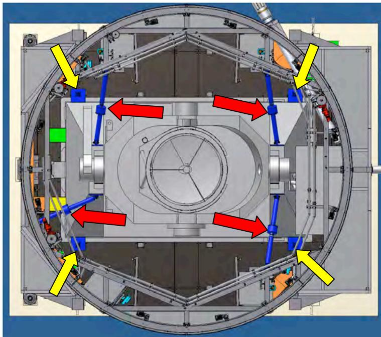
Fig 12. Dampers (yellow arrows) and stabilizing bars (red arrows)
