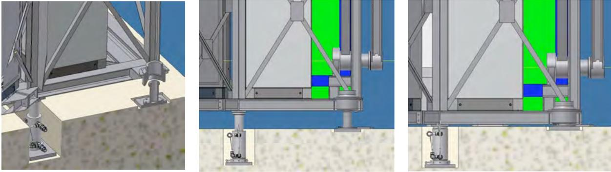
Fig 11. Isometric and side view of the hydraulic jack and UTE centring pin
