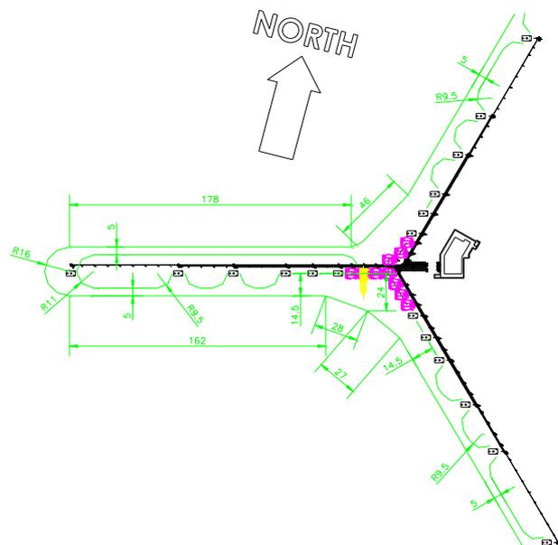
Fig 4. Relocation path along the array (green) based on reachstacker performances
