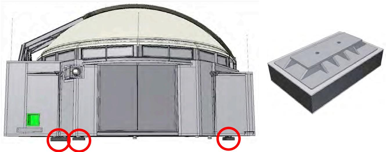
Fig 15. Safety pads mounted in correspondence of the UTE interfaces with the station
