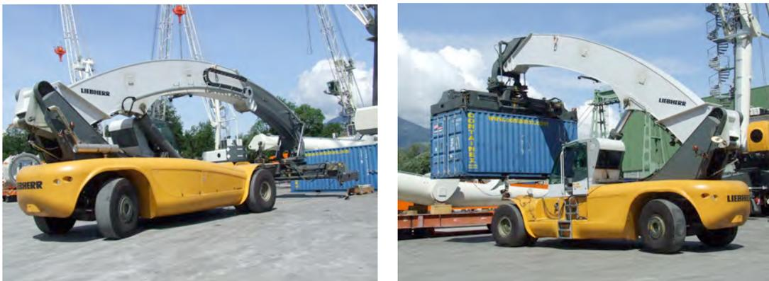
Fig 9. Reachstacker during tests without dummy (left) and with dummy load (right)
