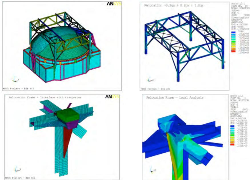
Fig 10. Relocation frame finite element analysis models and post processing
