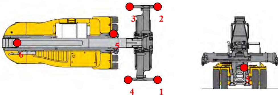
Fig 5. Accelerometer position during test performed
