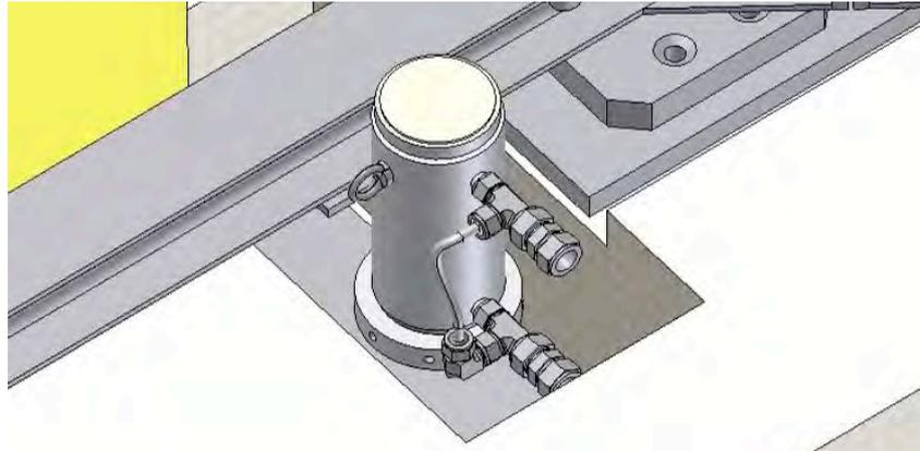
Fig 8. Hydraulic jack and insertion pit
