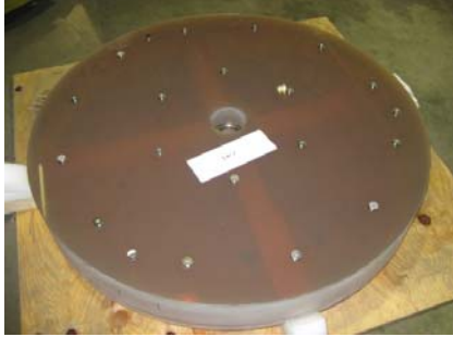
Figure 5: MROI 1.4 meter primary mirror. Courtesy of OST.
