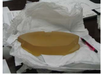
Figure 7: MROI 260 x110 mm flat tertiary mirror. Courtesy of OST.
