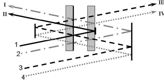
Figure 3. The pupil plane beam combiner P4. In this all-on-one scheme, the incoming beams (1 to 4) are recombined into the (I-IV) output beams which contains all interference between pairs.
