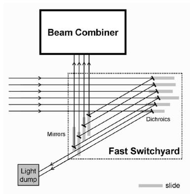
Figure 2. Schematic layout of the fast switchyard design. The 6 input beams enter horizontally from the left, while the 4 selected beams exit vertically. The beams transmitted by the dichroics exit to the right. The footprints of the mechanical slides are shown as gray rectangles.
