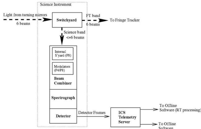
Figure 1. Block diagram of the near-infrared science instrument.
