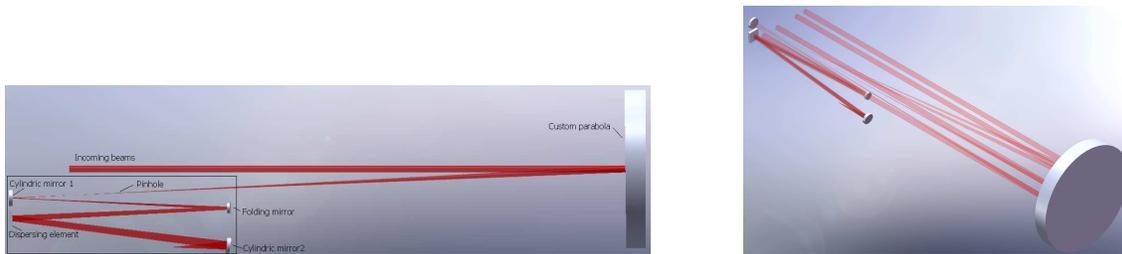
Figure 4. 3D views of the I4S design: from a plane perpendicular to the input beam configuration (left) and from the side (right).
