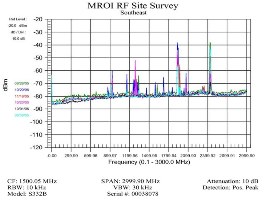
Figure 12: RF Survey with the horn antenna pointed in the Southeast direction with six sets of data.
