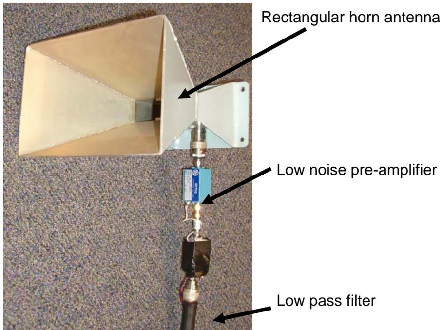
Figure 2: Horn antenna with a low noise pre-amplifier
