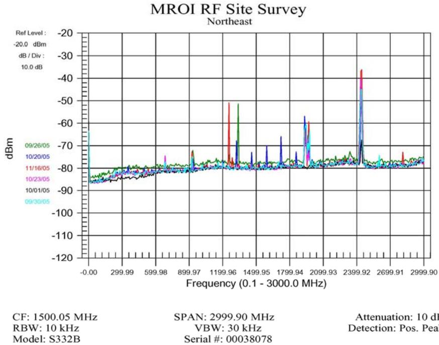
Figure 7: RF Survey with the horn antenna pointed in the Northeast direction with six sets of data.
