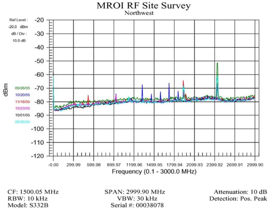
Figure 5: RF Survey with the horn antenna pointed in the Northwest direction with six sets of data.
