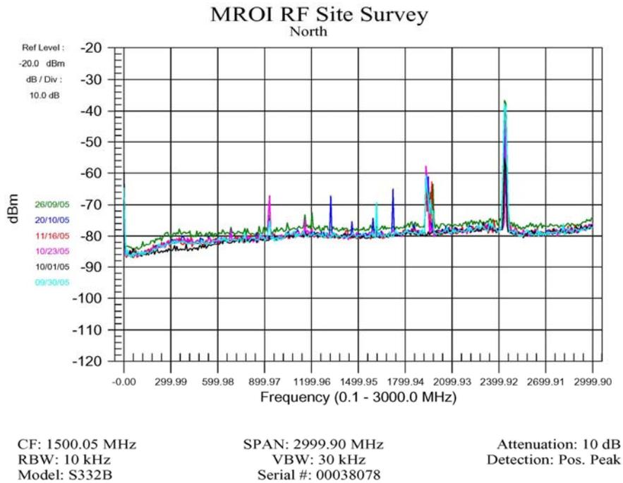
Figure 6: RF Survey with the horn antenna pointed in the North direction with six sets of data.
