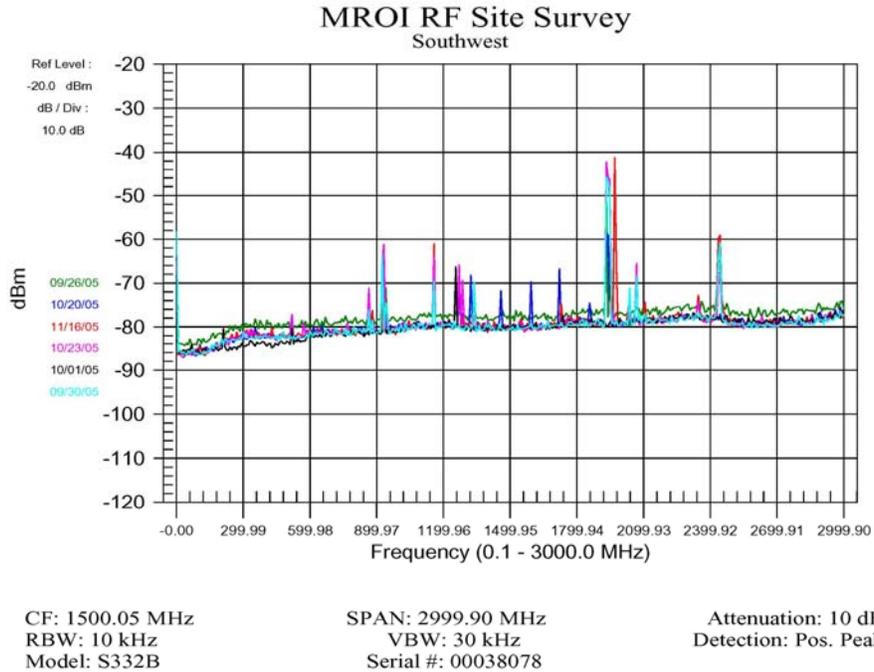
Figure 10: RF Survey with the horn antenna pointed in the Southwest direction with six sets of data.
