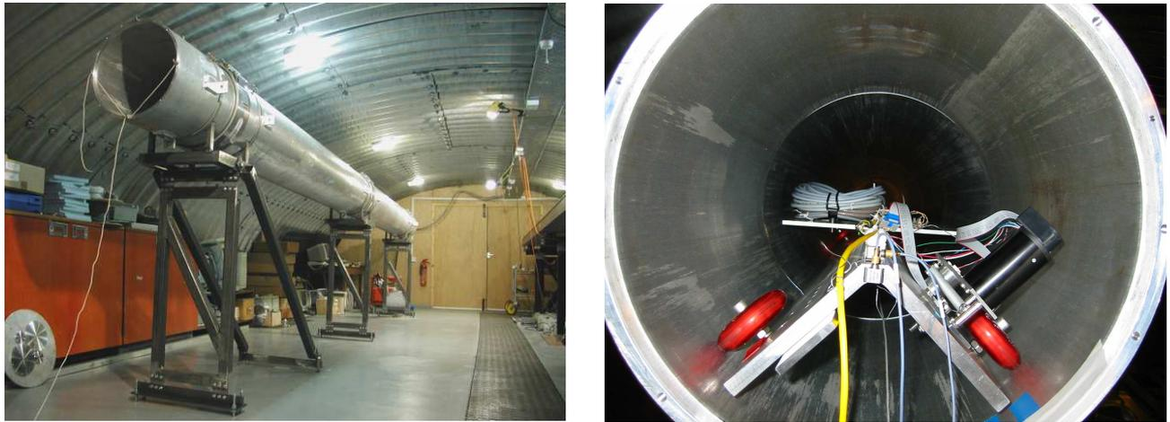
**Figure 8.** (Left) Photograph of the 7-metre-long test rig used for the risk reduction experiments. (Right) Photograph of the “embryo” trolley in the pipe test rig, showing the compliant wheels running at 45° to the vertical, the drive motor, and the cables for the accelerometers and other sensors.
