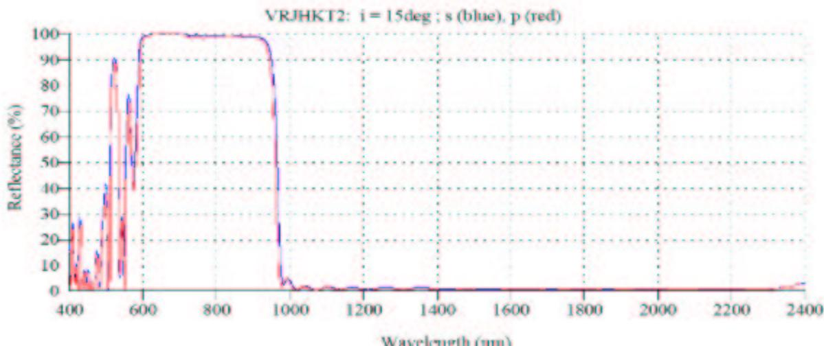
**Figure 4.** Newly designed multi-layer dichroic coating for MROI (see Hobson & Baldwin<sup>14</sup>). S and P polarizations overlay nearly exactly, indicating no difference in coating performance due to incident polarization.
