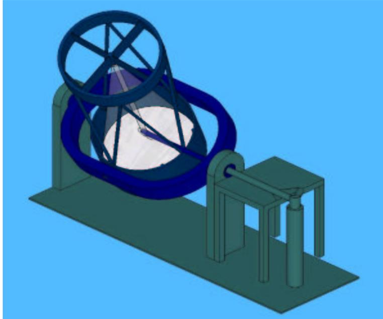
**Figure 3.** Altitude-altitude telescope design including optical table for the tip-tilt and ADCs.
