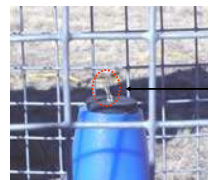
Figure 3 Thermocouple sticking out the end of a funnel.
