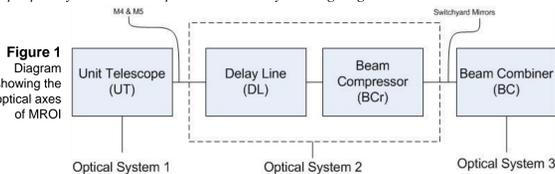
Depending on the location of the UT from start to finish the beam will travel distances ranging from 460 to 660 meters via several reflections that redirect the beam's path through the beam train into the delay line area (DLA) and finally into the beam combining area (BCA).
