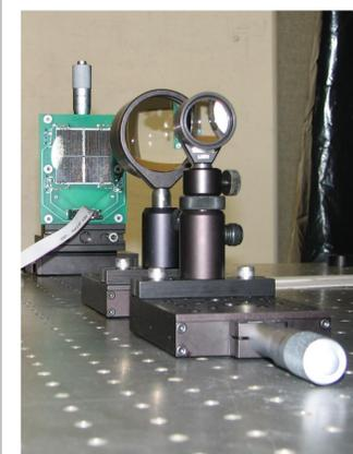
**FIGURE 8:** Photos showing the sketched test set up for the quad cells. A 78mm HeNe laser beam expanded 20x by a beam expander where it is then stopped down to 15mm beam by an iris and is diverted 45 degrees using a pellicle beamsplitter. It then travels through a pair of lenses which expands the beam to 30mm finally arriving at the quad cell. The quad cell is mounted on a x-y translation micrometer slide.
