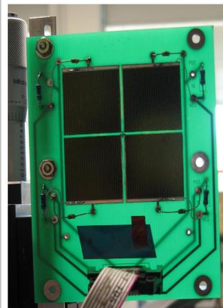
**FIGURE 6:** Custom made quad cell (50 x 50 mm) prototype
