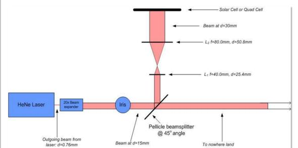
**FIGURE 7:** Sketch diagram of the lab set up for testing the quad cells.
