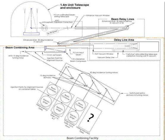
**FIGURE 2:** General optical layout of the beam's path from one unit telescope (UT) to the back end of the interferometer. Downstream a collimated beam exits UT at 95mm diameter, then propagates through the beam relay (BR) and the delay line (DL) pipes, finally entering the inner beam combining area (back end), where it first gets compressed by the beam reducer (BR) to 13mm diameter beam, before encountering the switchyard & the beam combining tables.
