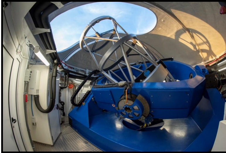
Figure 3: A fish-eye lens photograph inside a UTE looking at the UTM (see text for details). To the far right hand side one can see the inner edge of the Nasmyth platform. When moved, the entire assembly (UTM + UTE + UT optics (UTO) = UT) is moved as a single object, ideally using a reach stacker. Photo by Colleen Gino.
