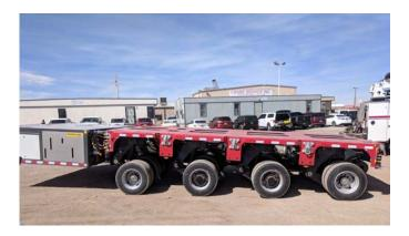
Figure 13 – Self-propelled Semi Trailer
