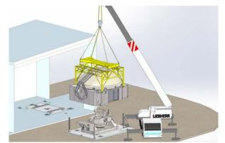
Figure 11 - 3D-CAD drawing of the UTE being integrated with UTM
