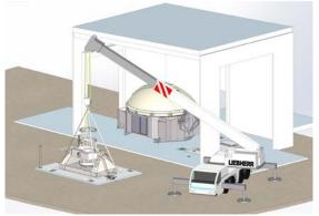
Figure 9 - 3D-CAD drawing of the UTM being lift it
