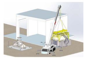
Figure 10 - 3D-CAD drawing of the UTE being lift it
