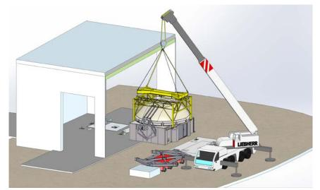
Figure 12 - 3D-CAD drawing of the UT being loaded on to the Transporter
