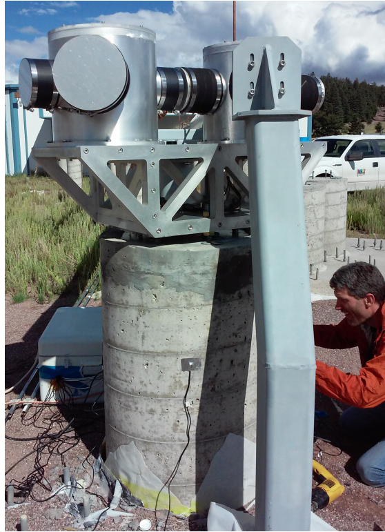
Figure 8: Beam relay vacuum can and support piers under test on MROI array.
