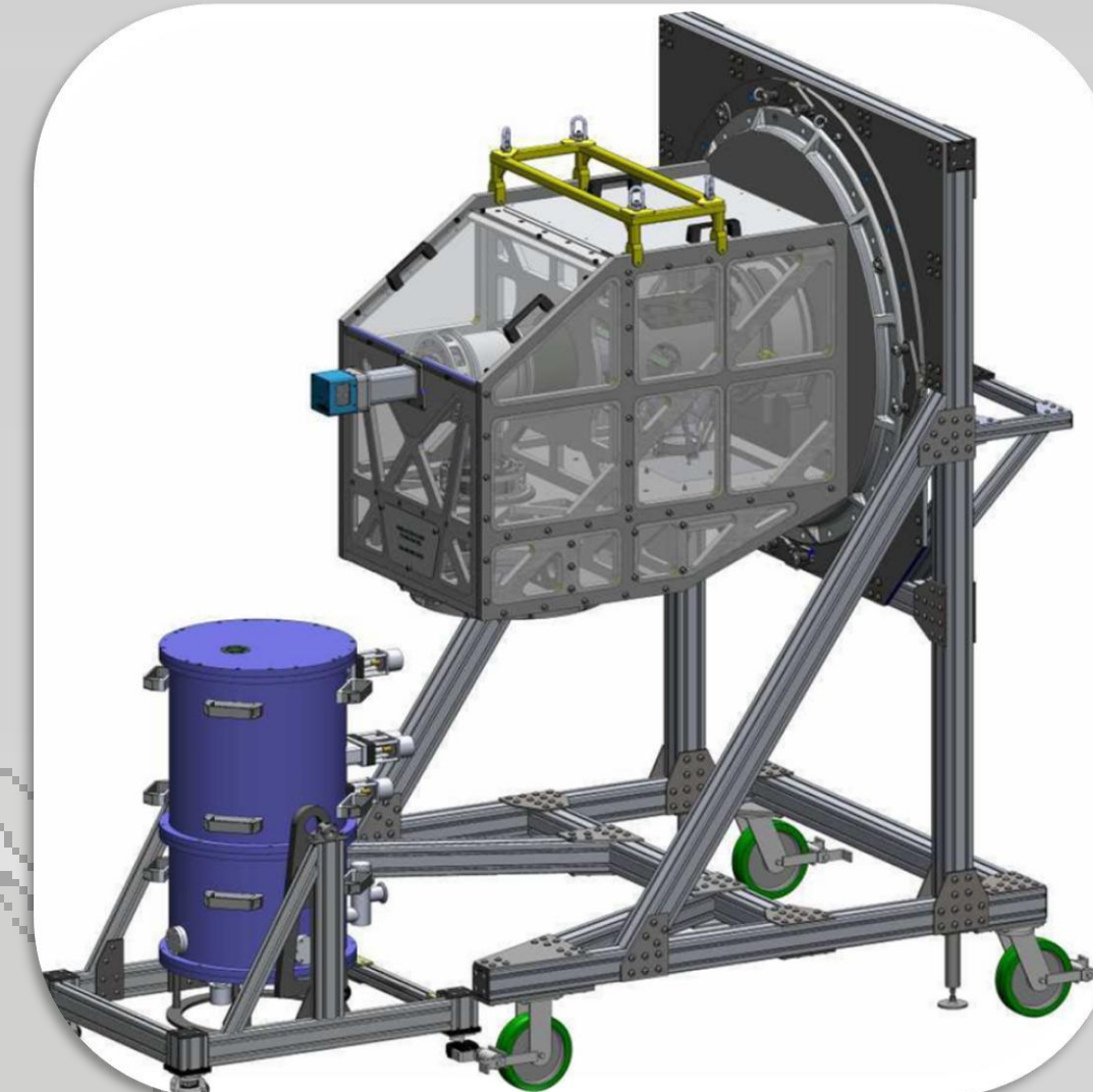
NESSI Handling and Testing Cart (right): This general purpose handling and testing cart will enable instruments to be mounted, integrated, aligned, and extensively tested in the lab, as well as facilitate assembly, handling, and servicing subassemblies at the telescope site.
