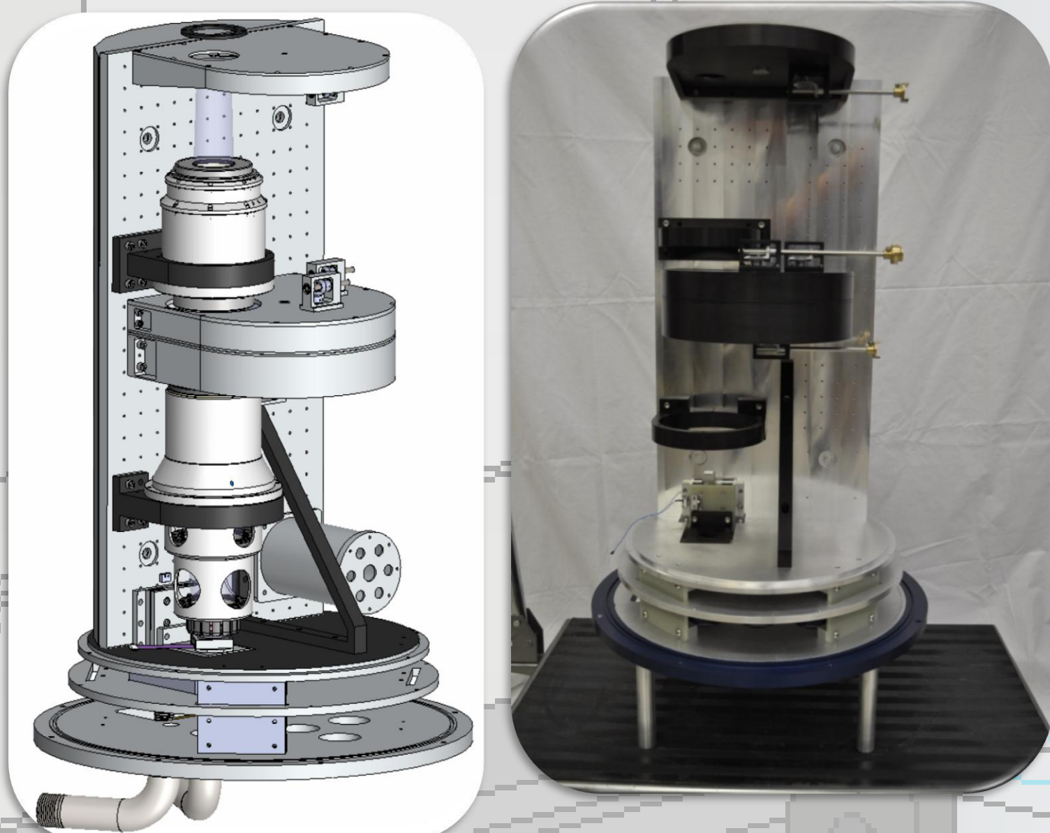
NESSI Dewar Spectrograph with Shields Removed Model (far left) and As Fabricated (near left): The collimator and camera barrels are assembled on angle brackets precisely mounted on the cold plate of the spectrograph.
