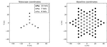
Figure 1 – MROI array layout (left) and instantaneous  $uv$  coverage (right) for a target at the zenith.
