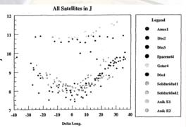
Measurements of infrared magnitudes of a number of GEO satellites from Sanchez et al (2000). In the H-band (1.6 micron wavelength) the objects were measured to be approximately 0.3-0.8 magnitudes brighter. The MROI with, an H-band limiting magnitude of 14, should be able to track fringes on all these targets, providing they have significant amounts of compact (<5m) structure.
