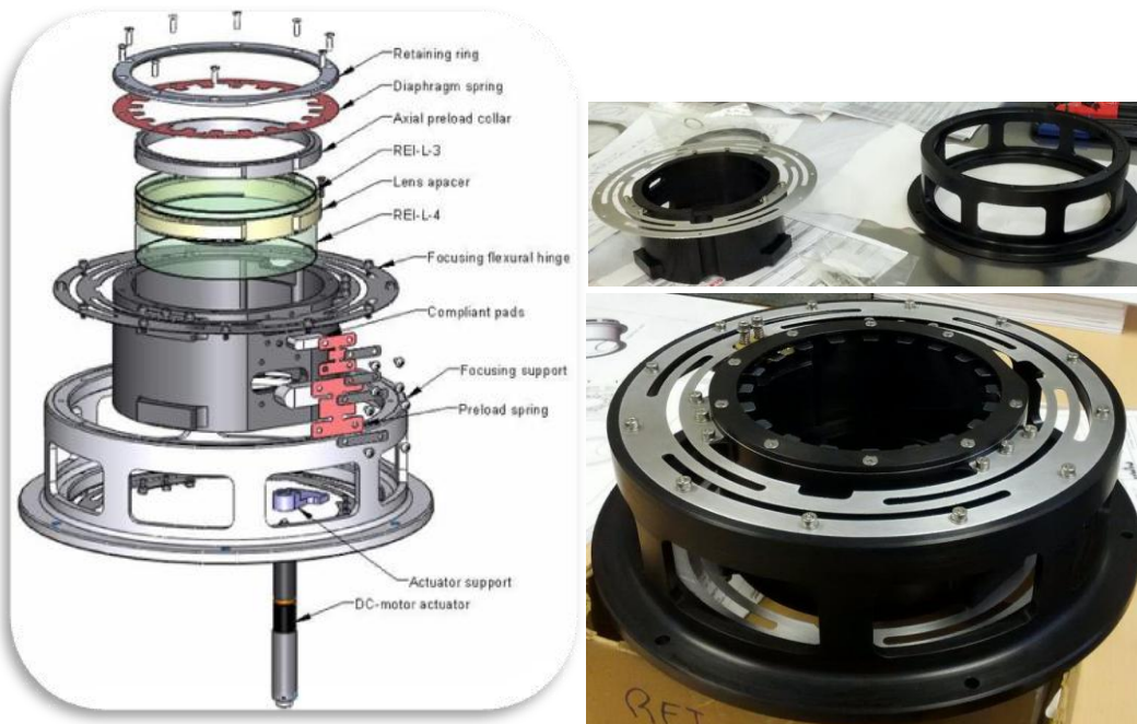
Figure 13 – NESSI re-imaging lens 3 and 4 - exploded view.
