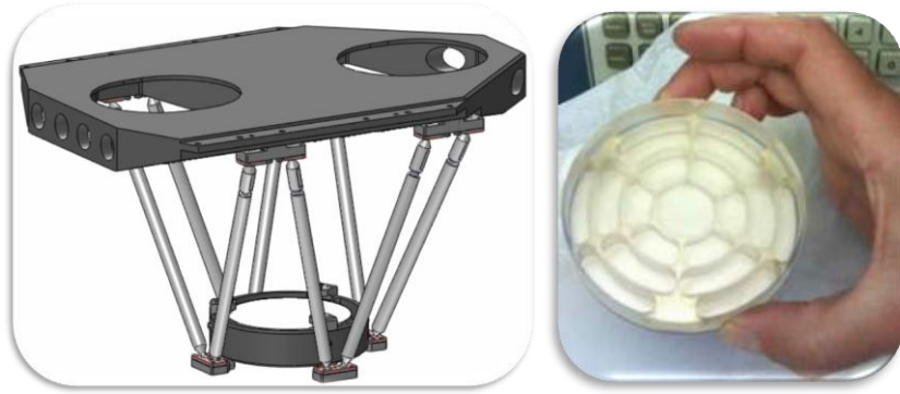
Figure 10 – NESSI KM-2 truss assembly and back of as-built mirror.
