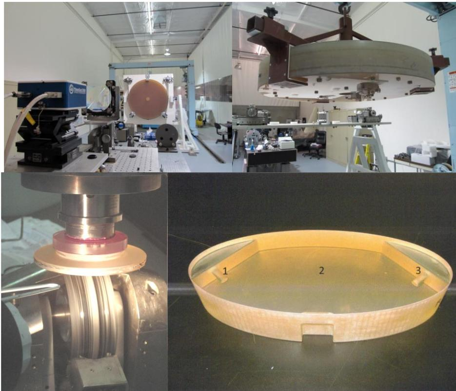
**Figure 4** - UTO (M1/M2/M3) - Top: The M1 SN1 primary at OST. Bottom left: The M2 mirror during polishing at QED. Bottom right: The M3 elliptical flat at OST.
