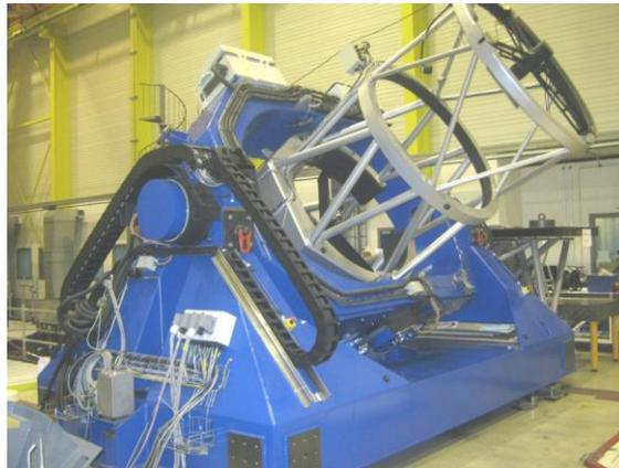
**Figure 2** - The MROI 1.4m UTM at AMOS facility during Factory Acceptance Test (Courtesy of AMOS).
