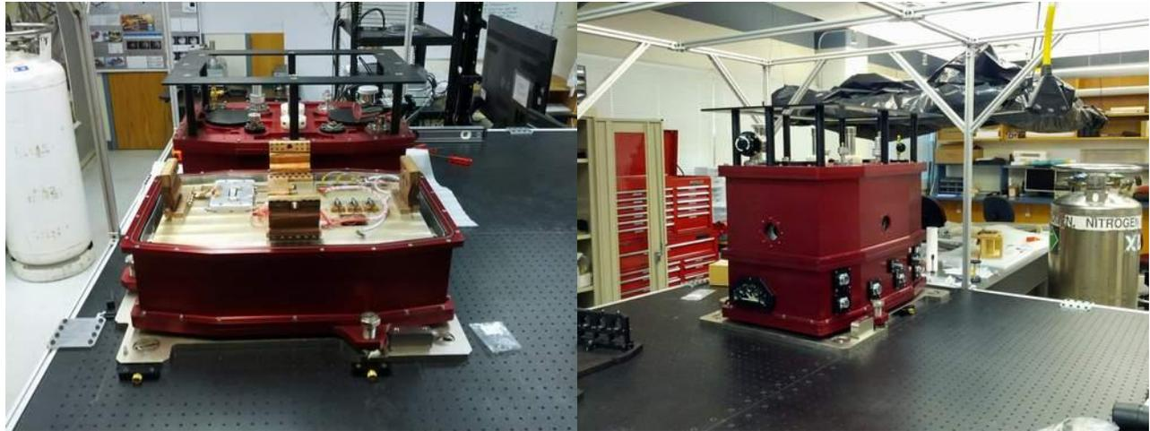
**Figure 20** - ICoNN spectrograph under assembly and testing.
