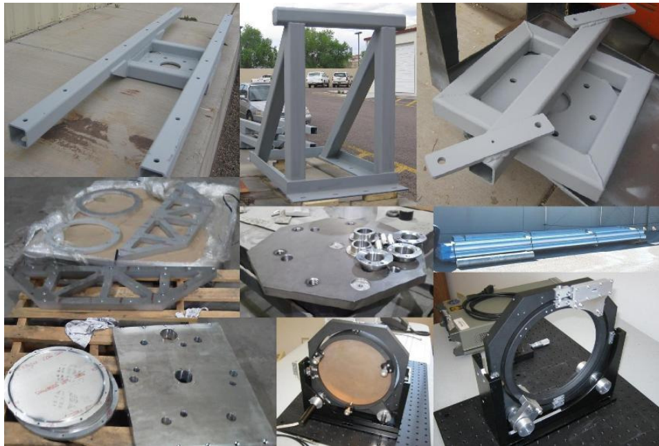
Figure 4: Components of the beam relay system under prototype and test in the lab and on-site at MROI.
