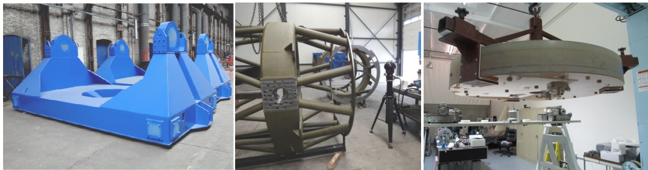
Figure 1: Telescope mounts and optics for the MROI: At left are the bases for UTs #2 and #3 at the AMOS factory; at center their corresponding two top ends; at the right UT #1's primary mirror is shown at the OST polishing facilities. Pictures are courtesy of AMOS and OST.
