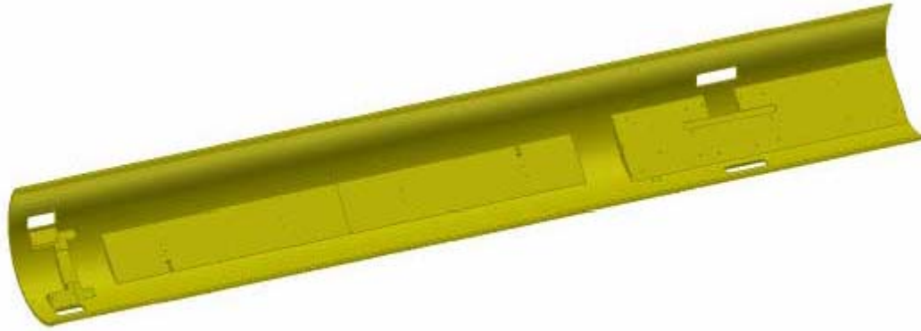
Figure 3. The trolley chassis has four separate segments glued into the half-cylinder. These are then machined in one operation to provide accurate location and alignment of the wheels and the cat's eye flexure mounts. Gaps between the segments are necessary to allow for the cat's eye primary mirror cell and secondary mirror structure.
