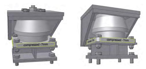
Fig 13. Damper with fixing plate and bracket
