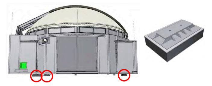
Fig 15. Safety pads mounted in correspondence of the UTE interfaces with the station
