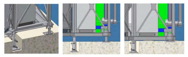
Fig 11. Isometric and side view of the hydraulic jack and UTE centring pin
