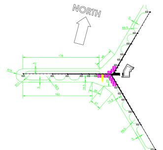
Fig 4. Relocation path along the array (green) based on reachstacker performances
