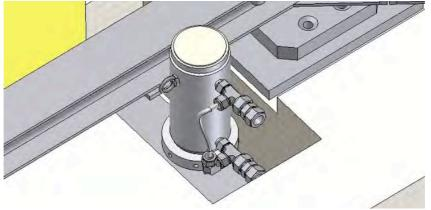
Fig 8. Hydraulic jack and insertion pit
