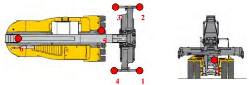
Fig 5. Accelerometer position during test performed
