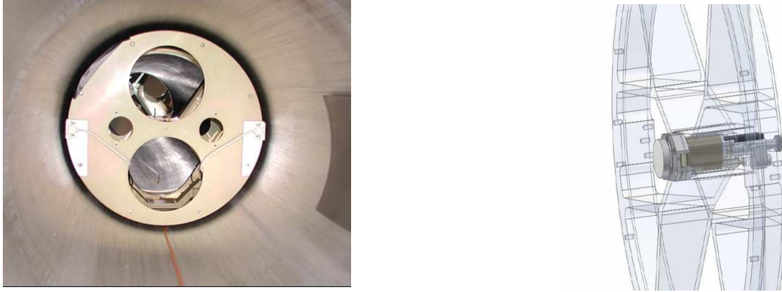
Figure 2. (Left) Photograph of the front face of the prototype delay line carriage travelling within the delay line vacuum pipe. The two large vertically spaced apertures show where the science beam enters and exits, while the smaller apertures to left and right show where the laser metrology beam passes. The lighter structures just outside the metrology beam apertures, to right and left, are the sensors that trigger when the carriage approaches the end of the vacuum pipe run. The wire used to supply power inductively to the carriage can just be seen running along the bottom of the pipe. (Right) CAD drawing of the details of the secondary mounting stage located at the front of the delay line carriage. The mounting and actuators for focus and tip-tilt control of the secondary are in the centre of the picture. This whole assembly is hidden behind the front entrance plate shown in the photograph to the left.
