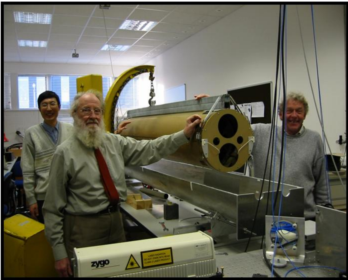
Figure 3. A delay line trolley is presented by three of our Cambridge collaborators during the Final Design Review in March, 2008. On the front of the cart one can clearly see where the stellar beams (top and bottom) and the metrology beams (left and right) enter the cat's eye assembly.
