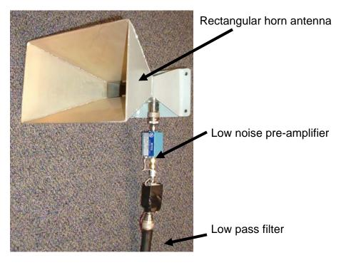
Figure 2: Horn antenna with a low noise pre-amplifier
