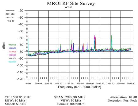
Figure 8: RF Survey with the horn antenna pointed in the West direction with six sets of data.
