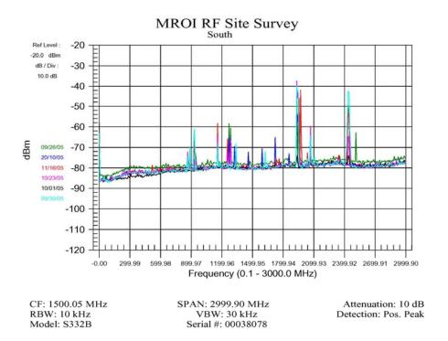
Figure 11: RF Survey with the horn antenna pointed in the South direction with six sets of data.
