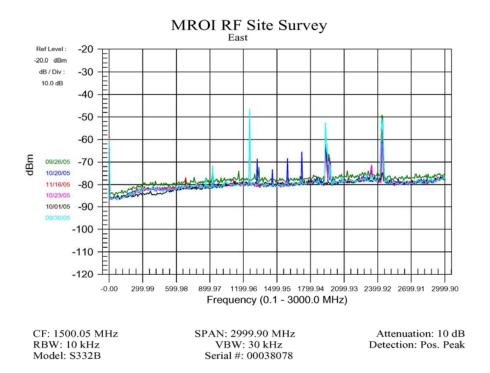
Figure 9: RF Survey with the horn antenna pointed in the East direction with six sets of data.
