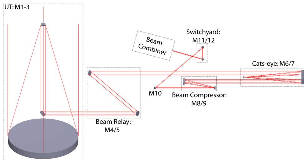
Fig. 2. Abbreviated optical train for a telescope on the west arm through to the first switchyard, illustrating the six optical assemblies.
