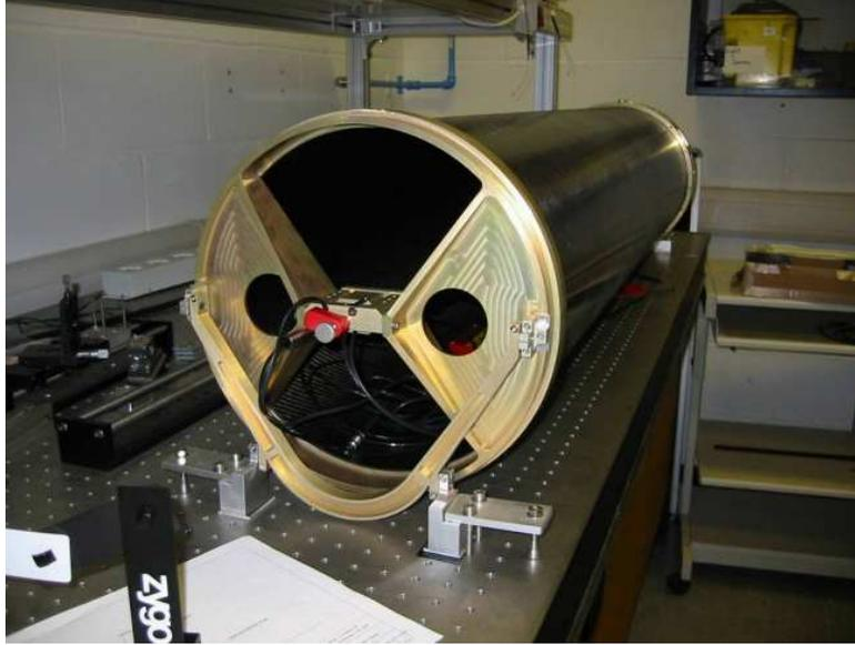
**Figure 7.** The Cat's-Eye assembly for the MROI delay line under test in the laboratory. The tube for the retroreflector is an approximately 1.2m in length and 30cm in diameter, and built from carbon-fiber reinforced plastic (CFRP) for stiffness.
