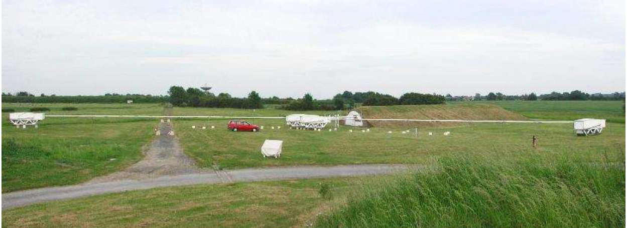
Figure 1. A view of COAST taken in June 2004. The maximum baseline, extending from the left hand North telescope to the right hand outer West telescope is roughly 67 m. Three of the 40 cm telescopes are clustered towards the center of the Y-shaped array, close to one end of the grass-covered beam combining laboratory. The station-wagon in the centre of the picture gives some sense of the scale.
