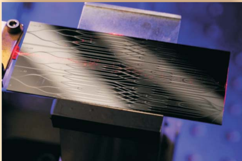
Figure 5. A beam combiner on a chip —an integrated-optics device manufactured using a silica-on-silicon process similar to the manufacture of integrated circuits—provides a large amount of optical processing power on a single small substrate. Integrated optics has been used in the communications industry for some time but is now being applied to interferometry. Optical components for splitting and combining beams are written into waveguides on the surface. The technology enables bulk optics that take up many square meters to be replaced by single chips smaller than a cell phone. (Courtesy of Laboratoire d'Astrophysique de l'Observatoire de Grenoble, CEA Leti, Université Joseph Fourier, and CNRS.)
